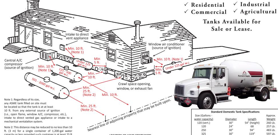
(i.e., open flame, window A/C, compressor, etc.), intake to direct vented gas appliance or intake to a mechanical ventalation system.
